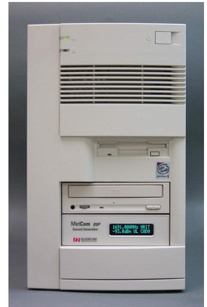
The MetCom DSP Second Generation Drivebay Receiver (rear panel inset) Typical PC mounting (right)
